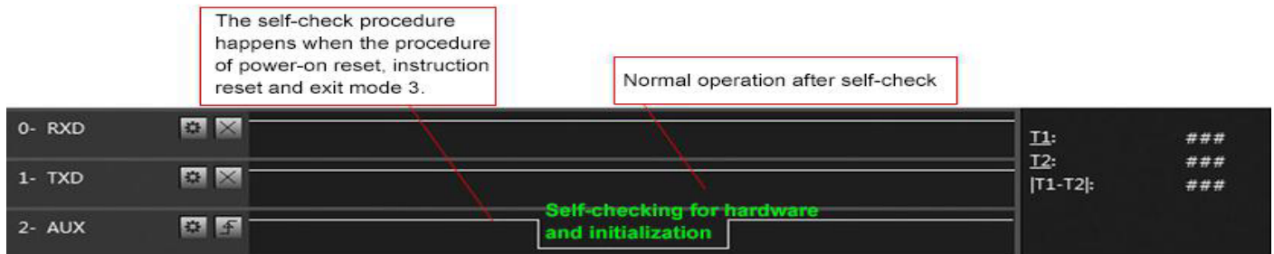
Timing Sequence Diagram of AUX when self-check
